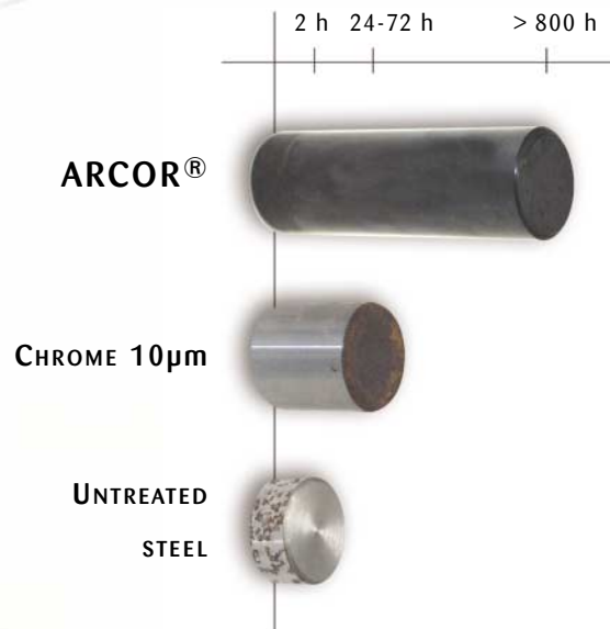
COMPARISON OF CORROSION RESISTANCE OF 41/40 STEEL WITH ARCOR® TREATMENT, WITH HARD CHROME COATING, AND WITHOUT TREATMENT
